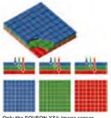
Only the FOVEON X3® image sensor captures 100% of the R(red), G(green), and B (blue) light at every pixel location.
