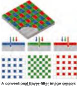
A conventional Bayer-filter image sensors capture only 25% of the R(red) and B(blue), and just 50% of the G(green).
